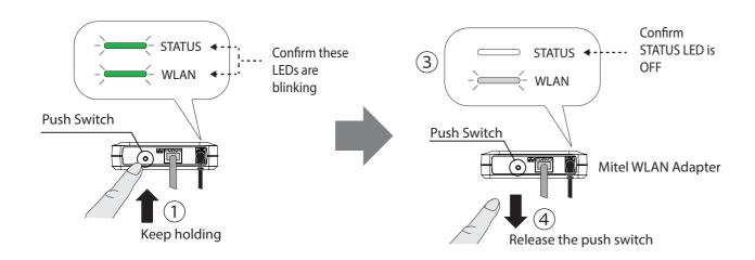
3 The Mitel WLAN Adapter will start to communicate with your wireless
