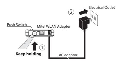
When the WLAN LED turns from Green to Red, release the switch. The factory default configuration is completed. After the factory default configuration is completed, the Mitel WLAN Adapter will restart.
